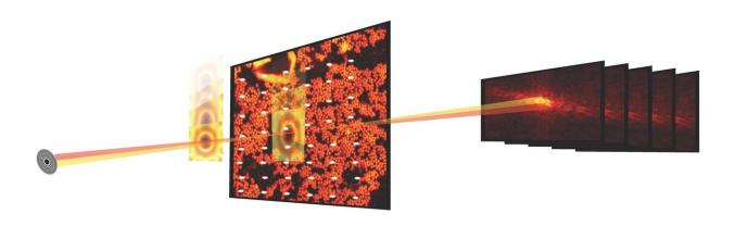
In scientific experiments, ptychographic imaging combines scanning microscopy with diffraction measurements to characterize the structure and properties of matter and materials. Advances in detectors and x-ray microscopes at light sources have made it possible to now measure a ptychographic dataset in seconds. Credit: Stefano Marchesini, Berkeley Lab
