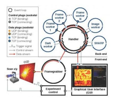
The modular, scalable Nanosurveyor II system—now up and running at the ALS—employs a two-sided infrastructure that integrates the ptychographic image data acquisition, preprocessing, transmission and visualization processes. Credit: Lawrence Berkeley National Laboratory
