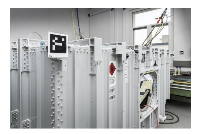
Through ambient markers on the tank the AR glasses know where the tank is and how large it is, allowing them to project a 3-D model. Credit: Markus Breig, KIT
