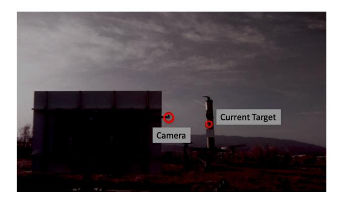
A digital camera mounted experimentally on a sample heliostat 'sees' the infrared light on the tower. Credit: CENER
