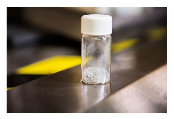
Army Research Laboratory scientists found that a nano-galvanic aluminum-based powder spontaneously splits hydrogen from water and liquids containing water without the need for a catalyst. Credit: US Army photo by David McNally
