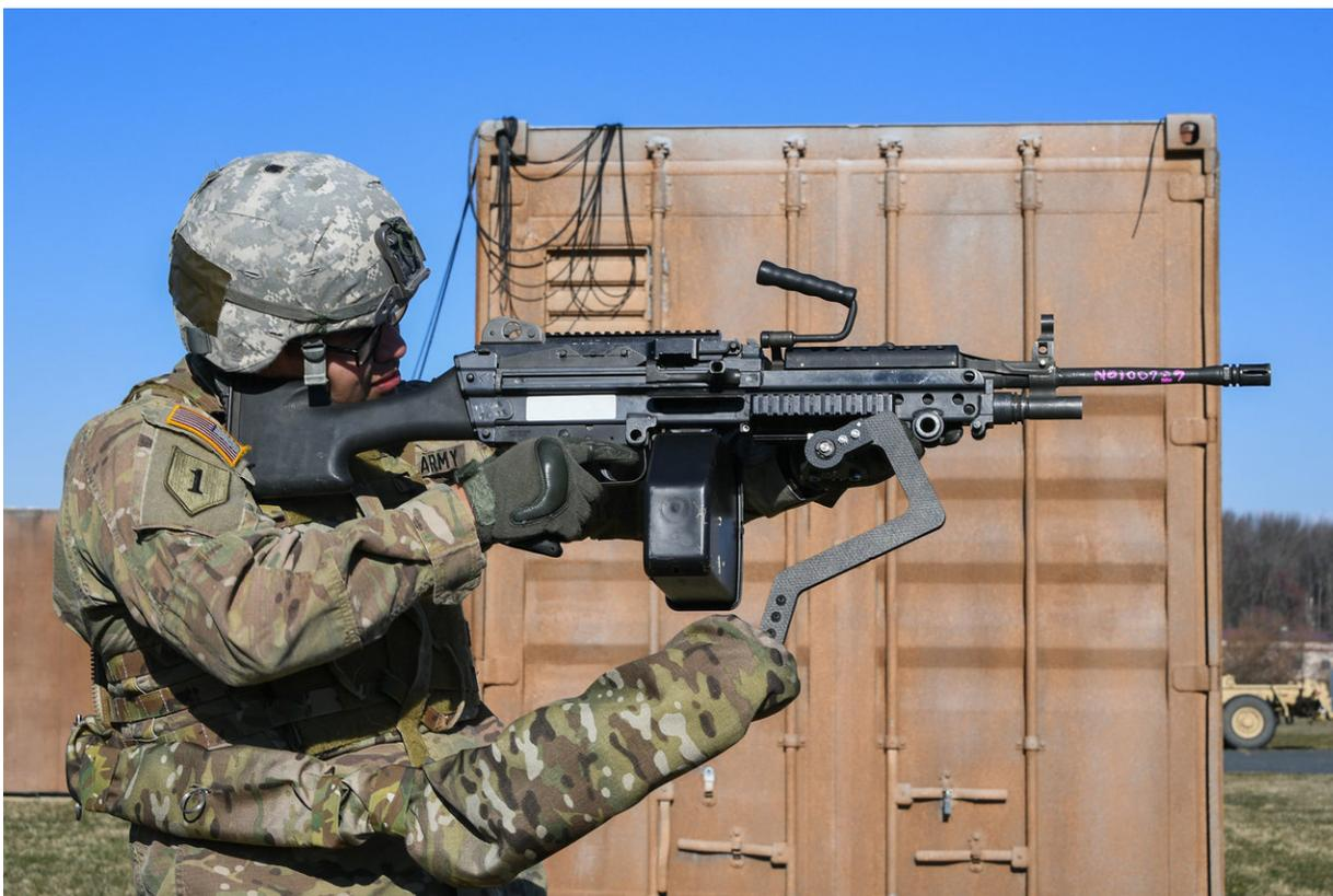
Army Sgt. Michael Zamora uses a prototype Third Arm exoskeleton to easily aim an 18-pound M249 light machine gun during testing at Aberdeen Proving Ground, Maryland, March 14, 2018. Credit: US Army photo by Conrad Johnson
