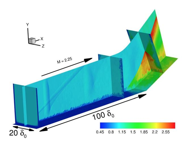
A simulation of supersonic turbulent flow on a ramp. Sharp lines show shock waves; irregular, smudged boundaries represent turbulent flow. Credit: Jonathan Poggie, Purdue University.
