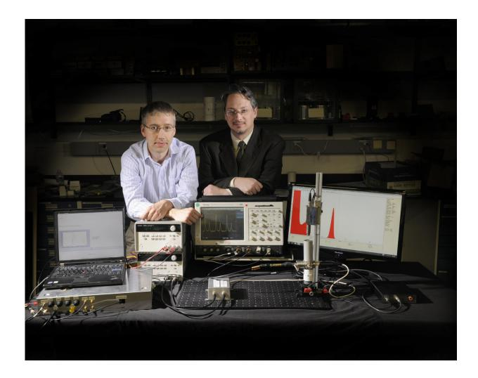
Engineers Luke Winternitz (left), Jason Mitchell (right) and their team developed a unique tabletop device -- aptly described as a 'pulsar on a table' -- to simulate rapid-fire X-ray pulsations needed to test algorithms and other advanced technologies for the X-ray navigation. The team recently delivered the special testbed to the Aeromechanics and Flight Mechanics Division's Electro-Optics Lab at the Johnson Space Center. Credit: NASA/P. Izzo
