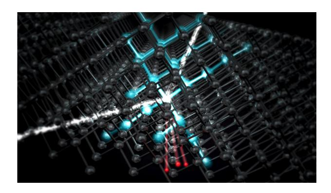
The future SuperCDMS SNOLAB experiment will hunt for weakly interacting massive particles (WIMPs), hypothetical components of dark matter. If a WIMP (white trace) strikes an atom inside the experiment's detector crystals (gray), it will cause the crystal lattice to vibrate (blue). The collision will also send electrons (red) through the crystal that enhance the vibrations. Credit: Greg Stewart/SLAC National Accelerator Laboratory
