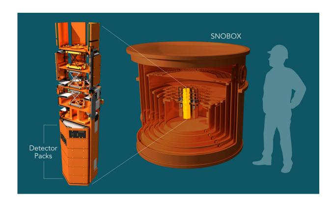
The centerpiece of the SuperCDMS SNOLAB experiment will be four detector towers (left), each containing six detector packs. The towers will be mounted inside the SNOBOX (right), a vessel in which the detector packs will be cooled to almost absolute zero temperature. Credit: Greg Stewart/SLAC National
