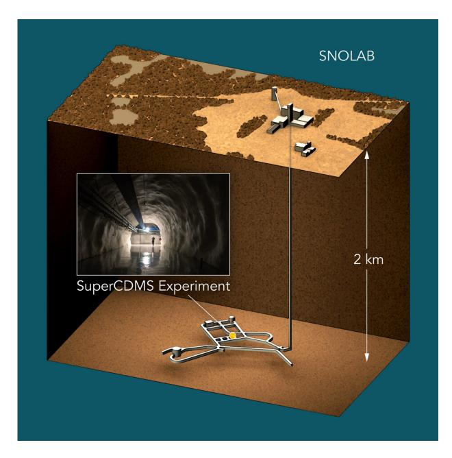
The SuperCDMS dark matter experiment will be located at the Canadian laboratory SNOLAB, 2 kilometers (6,800 feet) underground inside a nickel mine near the city of Sudbury. It's the deepest underground laboratory in North America. There it will be protected from high-energy particles, called cosmic radiation, which can create unwanted background signals. Credit: Greg Stewart/SLAC National Accelerator Laboratory; inset: SNOLAB
