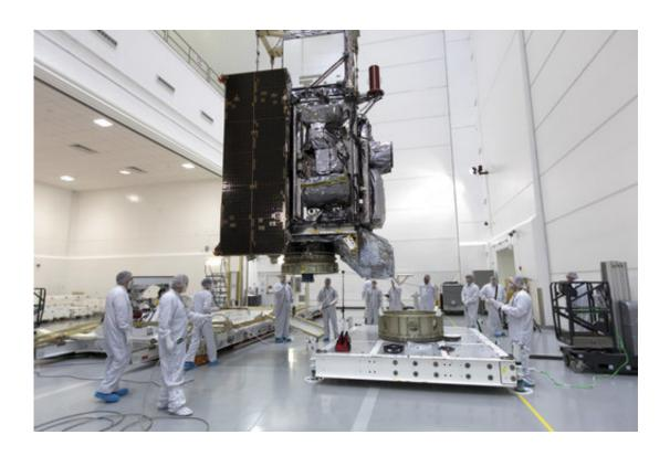
In this Dec. 6, 2017 photo made available by NASA, technicians and engineers move the National Oceanic and Atmospheric Administration's Geostationary Operational Environmental Satellite-S (GOES-S) to a work stand at Astrotech Space Operations in Titusville, Fla., near Kennedy Space Center. On Wednesday, May 28, 2018, NOAA said that the GOES-17's imager is not providing proper cooling for its infrared sensors. (Leif Heimbold/NASA via AP)
