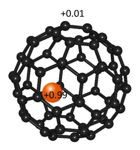
Calculated geometry and charges of LibC60[PF6 - ] salt. Credit: University of
