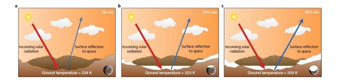
The simplified surface energy balance for early Mars showing the decrease in surface temperature with increasing amounts of surface ice. The resultant increase in surface reflectivity is represented by a widening blue arrow. Credit: Ramirez and Craddock (2018), *Nature Geoscience*
