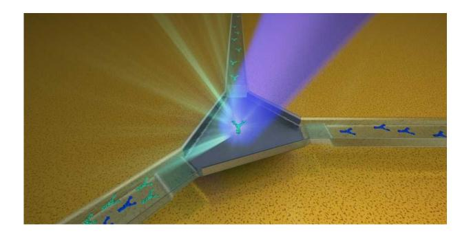
Graphical representation of a channel system with a junction and three valves, between which individual nanoparticles can be arrested. Credit: ETH Zurich / Giacomo Sebastiano Palamara
