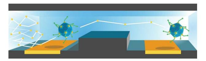
Schematic representation of a liquid-filled nanovalve in cross-section, through which a virus particle is transported. The bottleneck is depicted in the centre in grey, the electrodes in yellow. Credit: Eberle et al. Nature Nanotechnology 2018, edited
