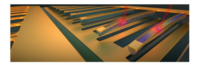
Electrodes stretch diamond strings to increase the frequency of atomic vibrations to which an electron is sensitive, just like tightening a guitar string increases the frequency or pitch of the string. The tension quiets a qubit's environment and improves memory from tens to several hundred nanoseconds, enough time to do many operations on a quantum chip. Credit: Second Bay Studios/Harvard SEAS
