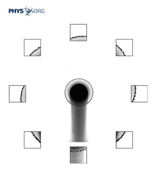
The MIT team released droplets onto a variety of surfaces, including onto the tip of a very thin rod, and captured droplets and ligaments flying off the rim during a single splash. Credit: Massachusetts Institute of Technology
