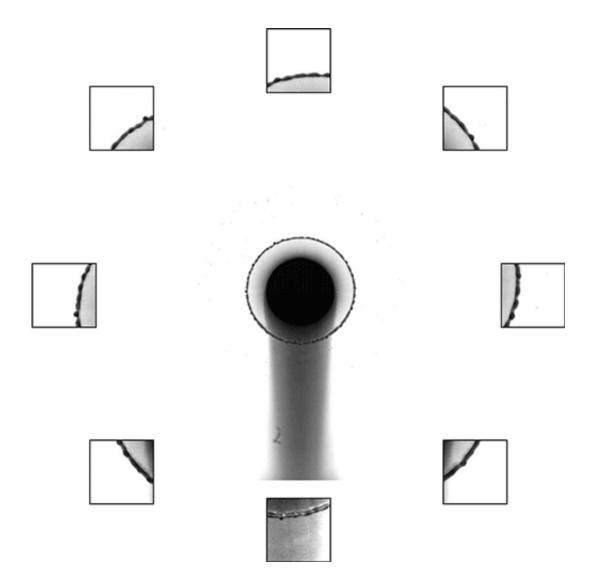
The MIT team released droplets onto a variety of surfaces, including onto the tip of a very thin rod, and captured droplets and ligaments flying off the rim during a single splash. Credit: Massachusetts Institute of Technology
