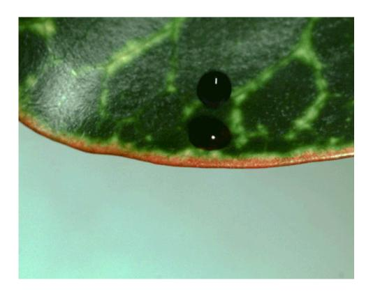
Measuring a droplet's rim can give scientists an understanding of how a single droplet can produce sprays when splashed on surfaces such as leaves. Credit: Massachusetts Institute of Technology
