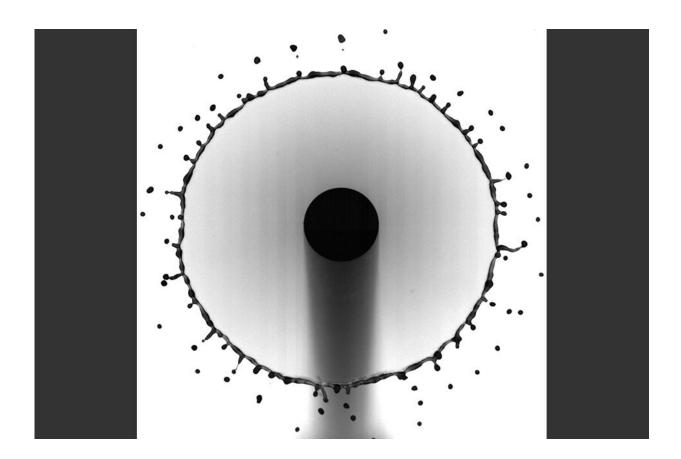
A droplet, splashing onto the tip of a very thin rod, produces a rim of fluid that sprays smaller droplets as it expands. Credit: Massachusetts Institute of Technology
