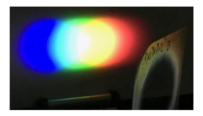
A one-inch diameter Bragg polarization grating diffracts white light from an LED flashlight onto a screen placed nearby. Even though the difference between the light's input and output direction is very large, the grating is highly efficient for a wide set of input angles. The extremely large color separation occurs because the grating structure has a nanoscale periodic structure smaller than the wavelength of visible light. Credit: North Carolina State University
