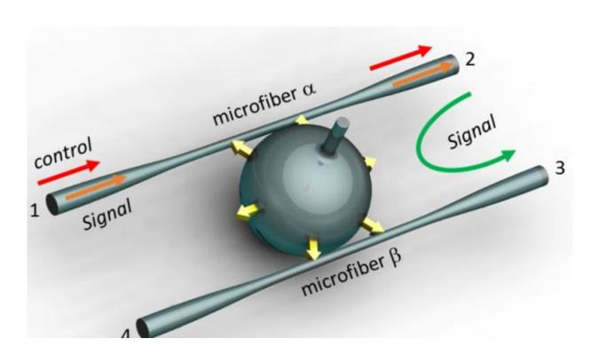
The schematic of the optomechanical circulator and directional amplifier designed by research group. Credit: SHEN Zhen
