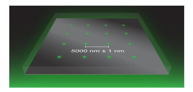
This illustration shows an array of apertures with a spacing of 5000 nanometers  $(nm) \pm 1$  nm. The apertures pass light through a metal film on a glass slide. Imaging the aperture array with an optical microscope results in apparent errors in the spacing between apertures. Knowledge of the true spacing allows correction of these imaging errors. This calibration process enables accurate measurements of position across a large image. Credit: NIST
