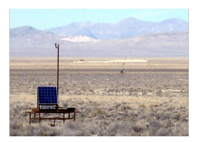
A Telescope Array Surface Detector and its neighbors, deployed in Utah's west desert. The 507 detectors are arranged on a grid covering 700 square kilometers, about the same as the land area of New York City. Credit: Telescope Array collaboration
