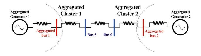
Synchronized cluster of an aggregated model obtained by simultaneously integrating the two sets of symmetrical generator groups and buss (connection point) groups in Figure 1. According to Ohm's law and Kirchhoff's law, it is a mathematically and physically feasible aggregated model. Credit: *Proceedings of the IEEE*
