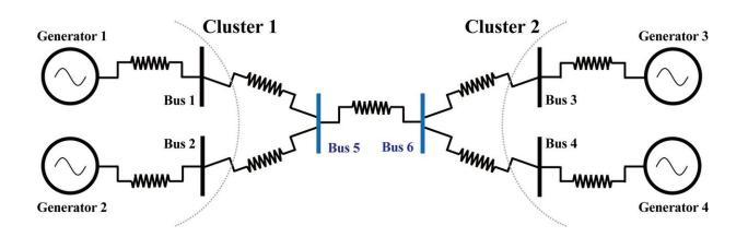
A power network consisting of four generators and six buses (connection points). Generators 1 and 2 and Buses 1 and 2 to which these are connected become a symmetrical network for Bus 5. Similarly, Generators 3 and 4 and Buses 3 and 4 become symmetrical for Bus 6. The two sets of symmetrical generator groups and buses are shown as Clusters 1 and 2. Credit: *Proceedings of the IEEE*
