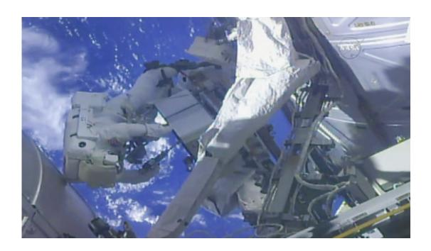
In this frame from NASA TV, NASA astronaut Ricky Arnold, left, and NASA astronaut Drew Feustel work on shuffling around a couple of space station pumps at the International Space Station on Wednesday, May 16, 2018. (NASA TV via AP)
