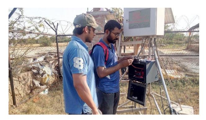
IITK researcher's Surya Gupta and Mithun Krishnan install thermal infrared radiometers to monitor land surface temperature at the critical zone observatory. Credit: Surya Gupta
