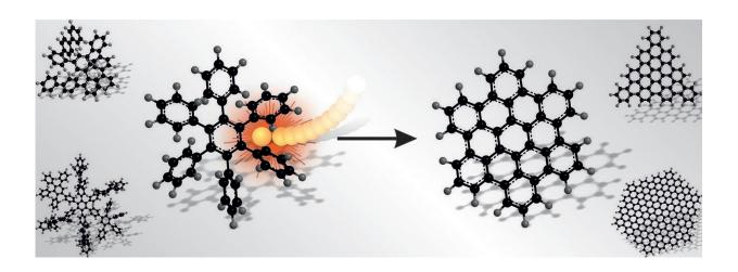
Mechanical energy provided by the collision of milling ball in planetary ball mills allows to synthesize nanographene structures under environmentally friendly and solvent-free reaction conditions. Credit: Sven Grätz
