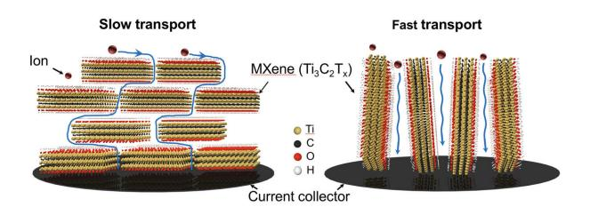
Soft assembly of MXene allows the 2-D materials to be stacked vertically, maintaining ion diffusion as the thickness of the material is increased. Credit: Drexel University
