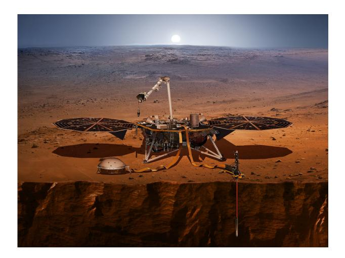
Artist's rendering of the InSight lander. The sensor assembly of the seismometer (underneath the protective shield) is pictured at the front left. Credit: NASA/JPL-CALTECH
