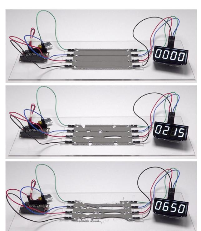
A digital clock continues to keep time as damaged circuits instantaneously heal themselves, rerouting electrical signals without interruption. Credit: *Nature Materials*
