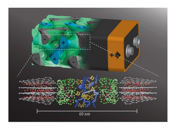
A rendering of the 3D battery architecture (top; not to scale) with interpenetrating anode (grey, with minus sign), separator (green), and cathode (blue, plus sign), each about 20 nanometers in size. Below are their respective molecular structures. Credit: Wiesner Group
