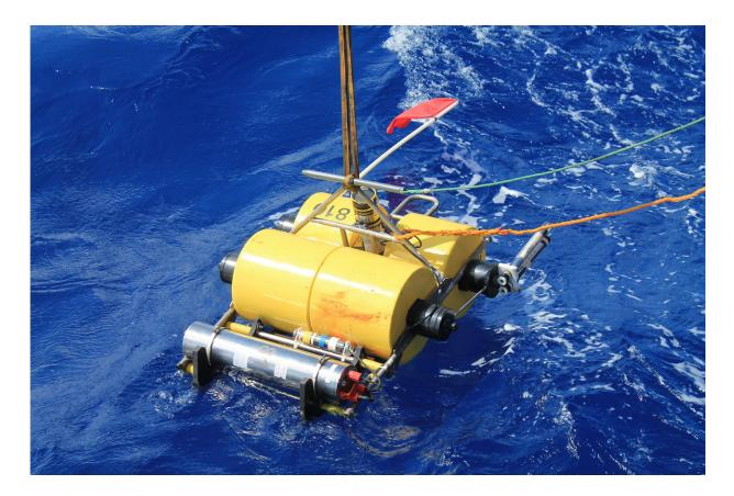
The launch of an ocean bottom seismometer. With these instruments record seismic waves at the sea floor. Credit: Ingo Grevemeyer/GEOMAR
