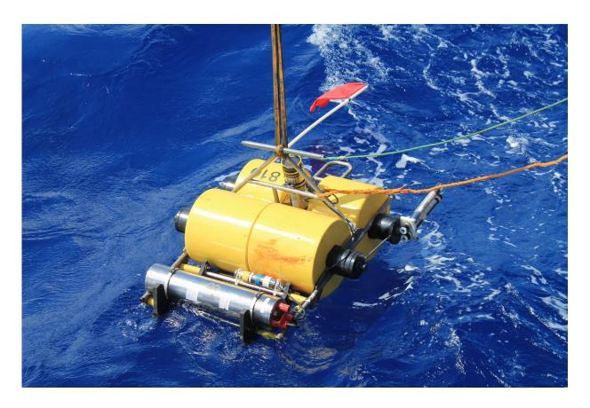
The launch of an ocean bottom seismometer. With these instruments record seismic waves at the sea floor. Credit: Ingo Grevemeyer/GEOMAR
