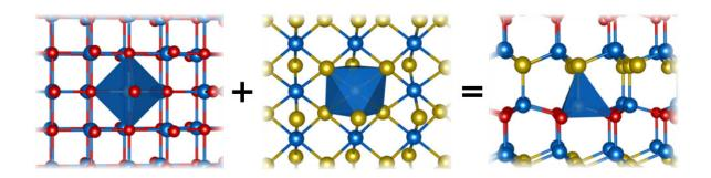
A team led by scientists at NREL demonstrated a way to use "negative pressure" to combine two dense materials into an alloy (right) with a much lower density, as if turning a snowball back into fluffy snow. The new alloy also has much different properties than either of its parents. The spheres represent atoms of manganese (blue), selenium (red) and tellurium (gold). Credit: SLAC National Accelerator Laboratory
