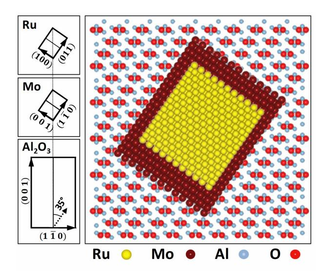
This schematic illustrates how a tetragonal phase of Ru has been forced using ultra thin film growth methods. Credit: University of Minnesota, Quarterman *et al, Nature Communications*
