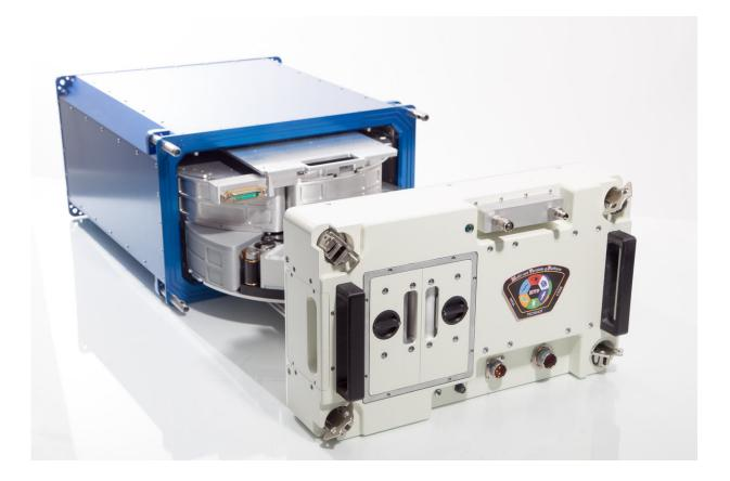
Two carousels sit inside MVP and can create up to 2 g of force. Each carousel can be set to spin at a different speed. Credit: Techshot
