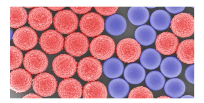
Rough and smooth particles in a suspension: Their mixing ratio influences the time of the sudden increase in viscosity. Credit: SEM image: Chiao-Peng Hsu, ETH Zurich
