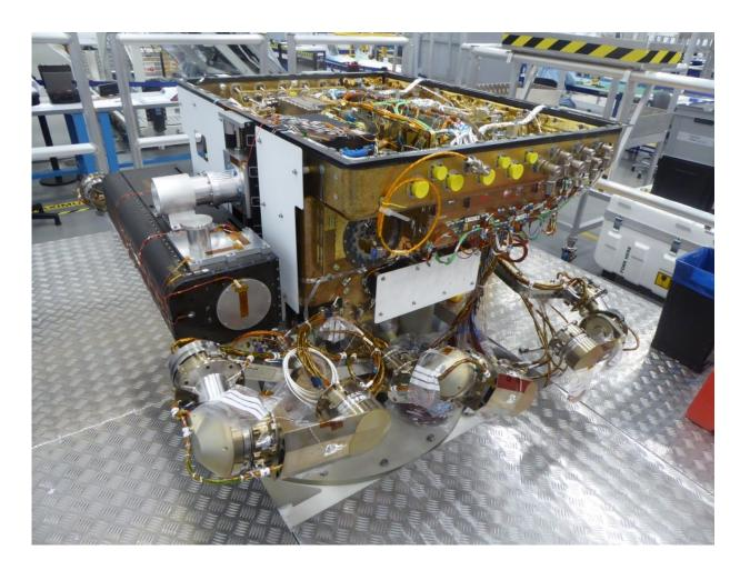
The structural model of the ExoMars rover, provided by ESA as part of the ESA/Roscosmos ExoMars mission, in which two out of the three wheel bogies can be seen facing the viewer. The black box towards the left is the drill box. The drill will be capable of accessing down to two metres below the surface to retrieve samples that may be better preserved against the harsh radiation experienced at the surface. Credit: Airbus Defence and Space UK
