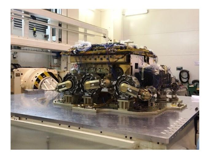
The structural model of the ExoMars rover, provided by ESA as part of the ESA/Roscosmos ExoMars mission, with three of its six wheels visible. In this configuration they are folded up against the rover body; they will be released after landing. The white panel towards the right is a radiator. The black square on the white panel is the inlet through which soil samples delivered by the drill will enter. Credit: Airbus Defence and Space UK
