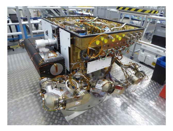
The structural model of the ExoMars rover, provided by ESA as part of the ESA/Roscosmos ExoMars mission, in which two out of the three wheel bogies can be seen facing the viewer. The black box towards the left is the drill box. The drill will be capable of accessing down to two metres below the surface to retrieve samples that may be better preserved against the harsh radiation experienced at the surface. Credit: Airbus Defence and Space UK
