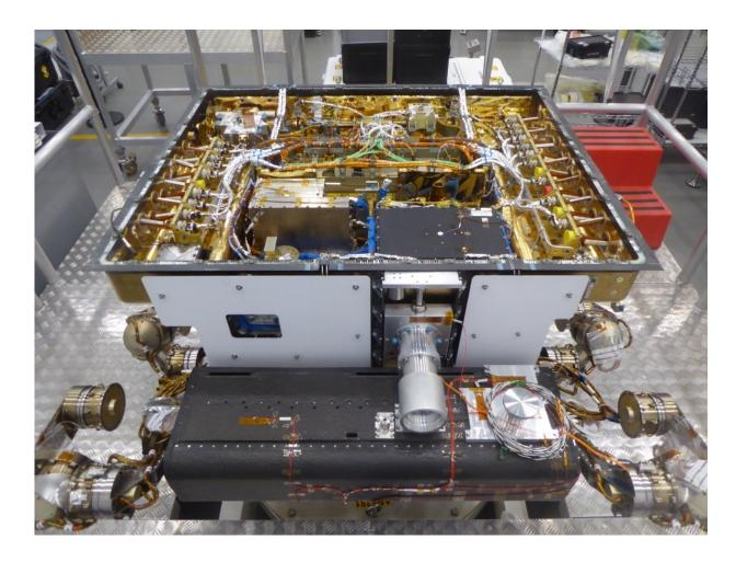
Front view of the structural model of the ExoMars rover, provided by ESA as part of the ESA/Roscosmos ExoMars mission. The black box at the front will contain the rover's drill, which will retrieve samples and deliver them to the onboard laboratory through the gap seen in the white panel at the front left. Credit: Airbus Defence and Space UK
