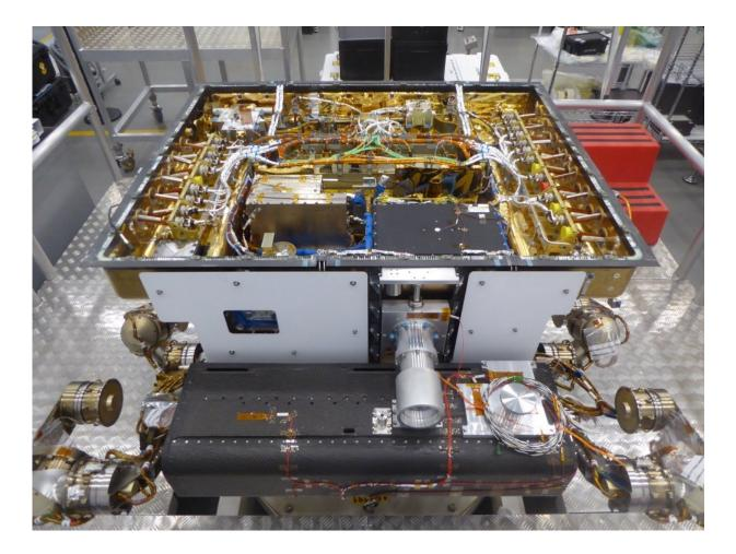
Front view of the structural model of the ExoMars rover, provided by ESA as part of the ESA/Roscosmos ExoMars mission. The black box at the front will contain the rover's drill, which will retrieve samples and deliver them to the onboard laboratory through the gap seen in the white panel at the front left. Credit: Airbus Defence and Space UK
