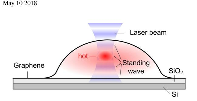
Bubbles form when molecules are trapped between the graphene sheet and the silica (SiO2/Si) substrate. The image shows also the hottest spot in red, which corresponds to the highest part of the bubble. Credit: Institute for Basic Science
