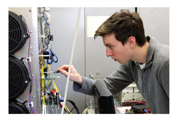
Colin Adams, a UW-Madison physics undergraduate, makes an adjustment to a novel prototype camera that will be used to image the fleeting signatures of gamma rays crashing into molecules of air in the Earth's atmosphere, creating a shower of diagnostic secondary particles. Credit: Savannah Guthrie
