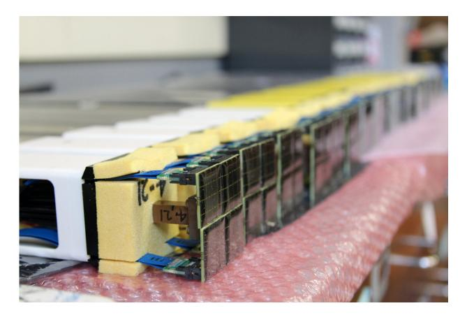
Sensors and electronic modules that are the heart of a prototype camera being integrated by UW–Madison physicists in support of the Cherenkov Telescope Array. The project is being facilitated by the Wisconsin IceCube Particle Astrophysics Center. Credit: Savannah Guthrie
