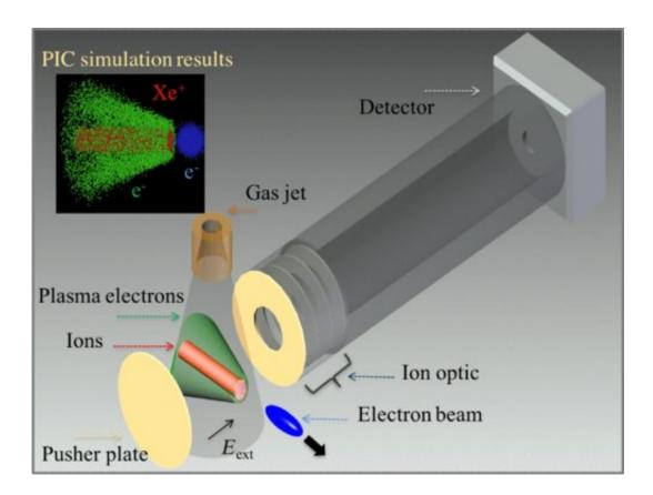
This diagram shows the setup for the proposed diagnostic, which includes a gas jet, an ion optic, and a detector. Credit: R. Tarkeshian, J.L. Vay, et al., *Phys. Rev. X* 8, 021039
