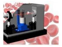
The laser beam passes through the blood sample and hits the detector on the other side. Two measurements are taken: one with the magnet next to the sample and one without the magnet. If there is any hemozoin in the blood, it will be pulled to the side of the sample holder by the magnet, changing the amount of light that can make it to the detector. Credit: Samantha McBirney
