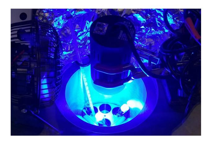
The setup of the photoredox polymerization in the glove box with a cold trap, irradiated by the blue LED light. Credit: Virginia Tech
