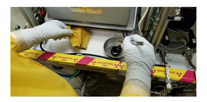
Scientists melt radioactive waste into glass in a test platform at PNNL designed to mimic Direct Feed Low-Activity Waste system being constructed at the Hanford, a former weapons production site in Washington State. Credit: PNNL
