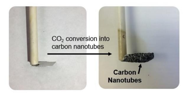
Small diameter carbon nanotubes grown on a stainless steel surface. Credit: Pint Lab/Vanderbilt Univerity
