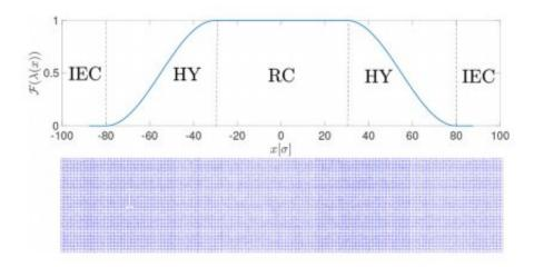
Setup of an adaptative resolution simulation for solids. Credit: Springer
