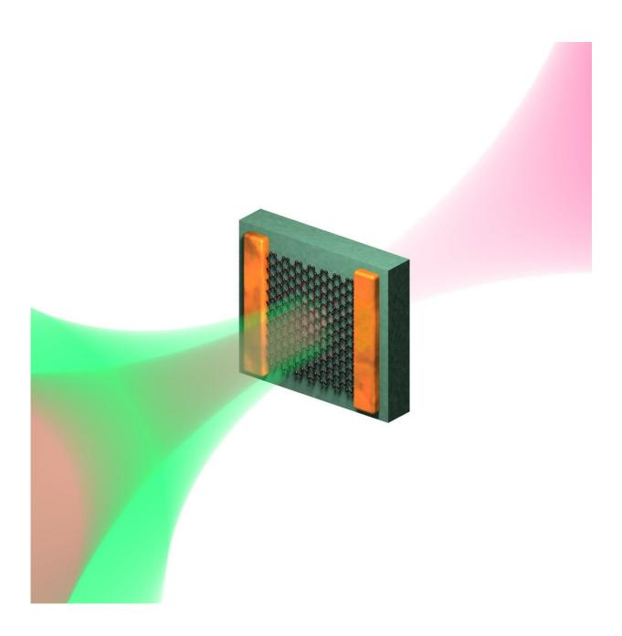
Schematic representation of the ultrafast optical pump - terahertz probe
