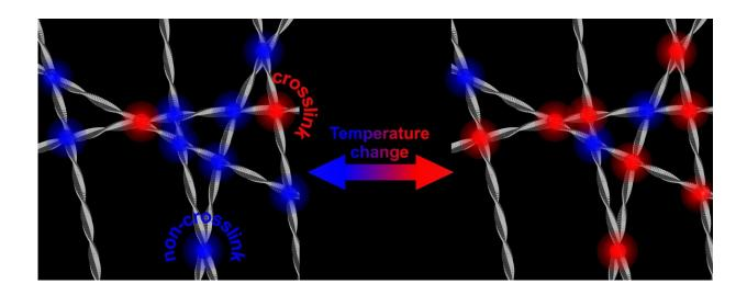
At higher temperatures, there are more crosslinks stiffening the network of protein fibrils. Lowering temperature results in a network that is less stiff again. Credit: University of Twente
