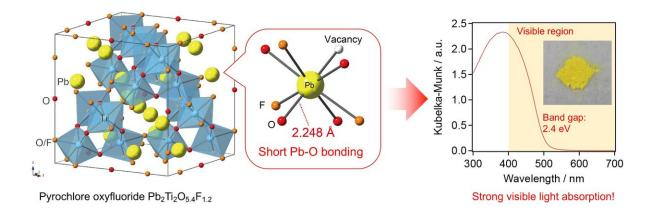
The inset shows an image of  $Pb_2Ti_2O_{5.4}F_{1.2}$ , shown to be capable of absorbing visible light of a wavelength of around 500 nm. This ability is thought to be due to the bonding structure around the Pb cation within the pyrochlore lattice, shown on the right. Credit: *Journal of the American Chemical Society*
