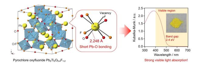
The inset shows an image of Pb<sub>2</sub>Ti<sub>2</sub>O<sub>5.4</sub>F<sub>1.2</sub>, shown to be capable of absorbing visible light of a wavelength of around 500 nm. This ability is thought to be due to the bonding structure around the Pb cation within the pyrochlore lattice, shown on the right. Credit: *Journal of the American Chemical Society*
