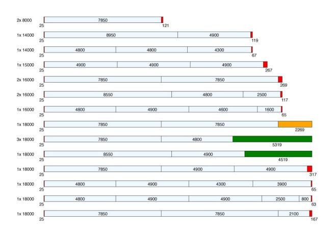
AutoBarSizer calculated cutting plan with leftovers. Green: reusable remainder (type 2), yellow: reusable remainder (type 1), red: scrap. Credit: Fraunhofer SCAI
