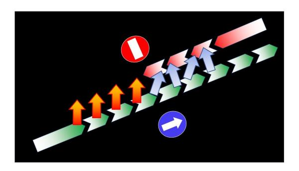
Spin chain in which spin interactions are strong in the left half (orange arrows) and weak in the right half (blue arrows). A spin current from left to right (green arrowed line) is possible, but not in the opposite direction (red arrowed line). A very large rectification is the result of this. Credit: SUTD
