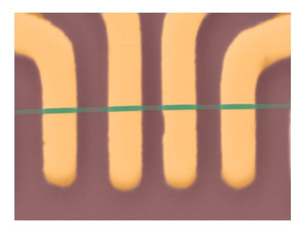
Microscopy image of an electronic device made with 1D ZrTe3 nanoribbons. The nanoribbon channel is indicated in green color. The metal contacts are shown in yellow color. Note than owing to the nanometer scale thickness the yellow metal contacts appear to be under the green channel while in reality they are on top Credit: Balandin lab, UC Riverside
