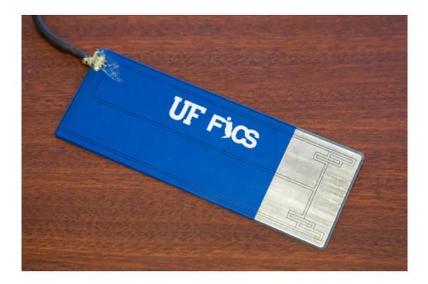
In this April 18, 2018 photo, a detection device under development by the University of Florida's Institute for Cybersecurity Research is displayed at the office of the New York Police Department's Financial Crimes Task Force. The device is slipped into a credit card reader and can detect if a skimmer device is present. (AP Photo/Mark Lennihan)
