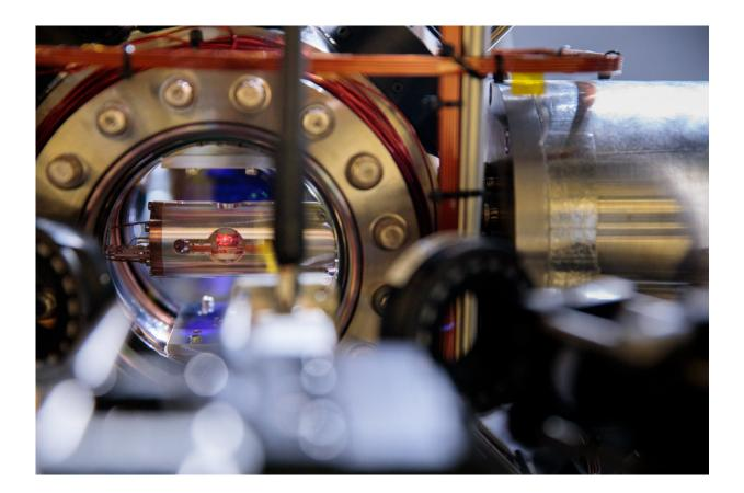
Look into the heart of an atomic clock. Here, a single atom is trapped in the metal vacuum chamber with the round window. The clock's tick comes from a laser tuned to interact with this atom. Credit: Centre for Quantum Technologies, National University of Singapore
