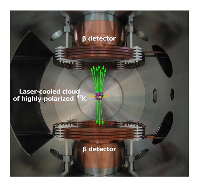
The measurement chamber of the TRIUMF Neutral Atom Trap (TRINAT)
