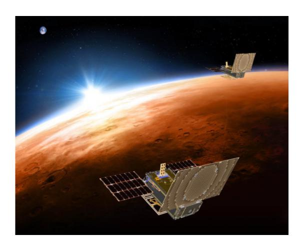
This illustration made available by NASA on March 29, 2018 shows the twin Mars Cube One (MarCO) spacecraft flying over Mars with Earth and the sun in the distance. The MarCOs will be the first CubeSats - a kind of modular, minisatellite - flown into deep space. They're designed to fly along behind NASA's InSight lander on its cruise to Mars. (NASA/JPL-Caltech via AP)
