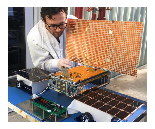
In this undated photo made available by NASA on March 29, 2018, engineer Joel Steinkraus uses sunlight to test the solar arrays on one of the Mars Cube One (MarCO) spacecraft at NASA's Jet Propulsion Laboratory in Pasadena, Calif. The MarCOs will be the first CubeSats - a kind of modular, mini-satellite - flown into deep space. They're designed to fly along behind NASA's InSight lander on its cruise to Mars. (NASA/JPL-Caltech via AP)
